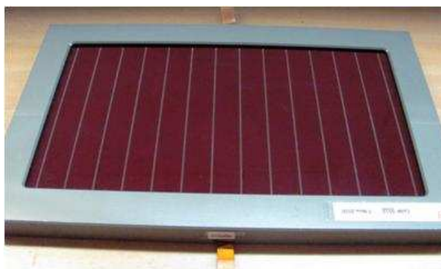
Figure 5.3 A double glass-substrate single cell from 3GSolar.
