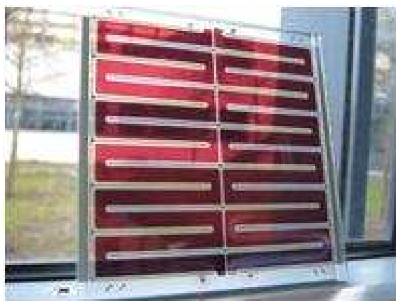
Figure 5.1. A 10 \times 10 \text{ cm}^2 current-collecting double glass-substrate sandwich devices from ECN /Fraunhofer ISE.
